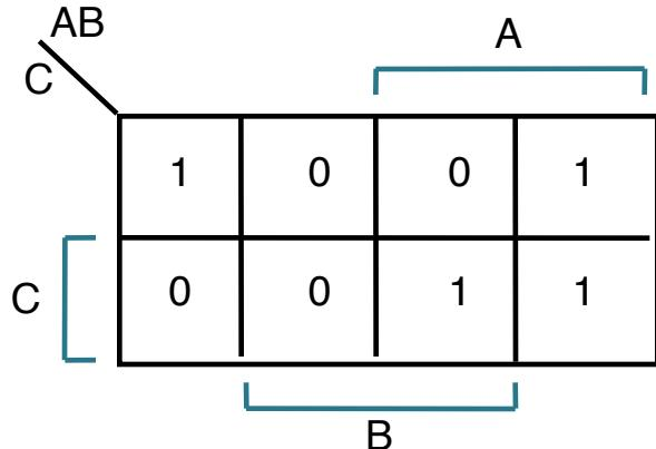
$$F(A,B,C) = \bar{A} \bar{B} \bar{C} + A \bar{B} \bar{C} + A \bar{B} C + A B C$$
